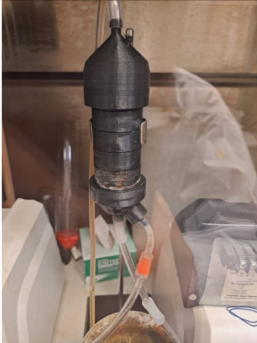
Figure 9 - 3D Printed Fixed Bed Treatment Column with Removable Cartridges
