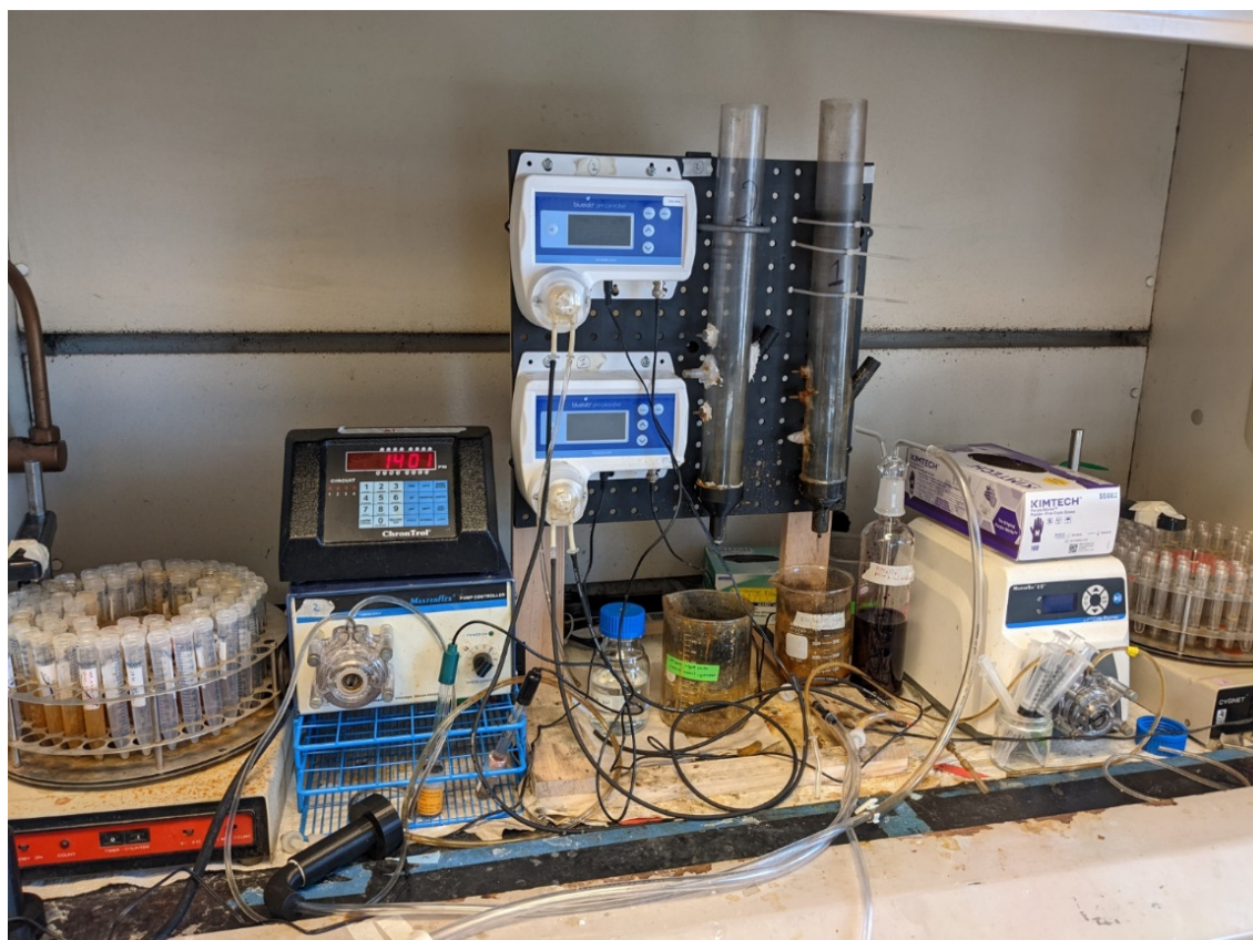
Figure 10 - Autosampler, peristaltic pump, timing control unit, pH controller, and column reactors (columns 1 and 2) used for ME experiments
