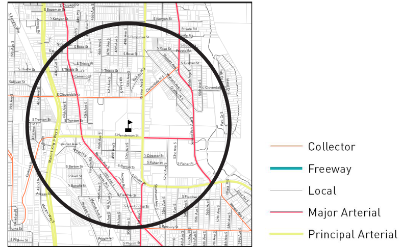
Figure 5.6: Comparison of road hierarchies within a 1-mile walkshed of South Shore K-8 (Source: Author)
