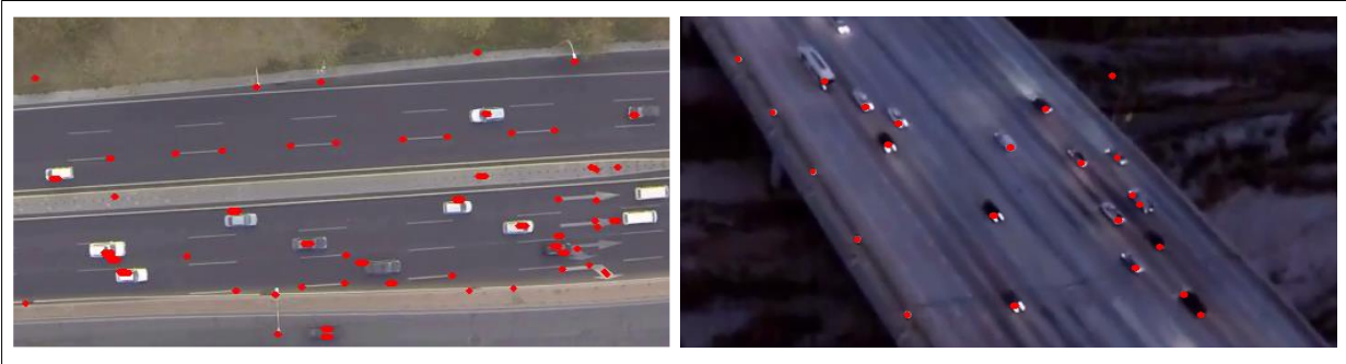
Figure 6-6 Two snapshots showing the interest points extracted in daytime and nighttime
