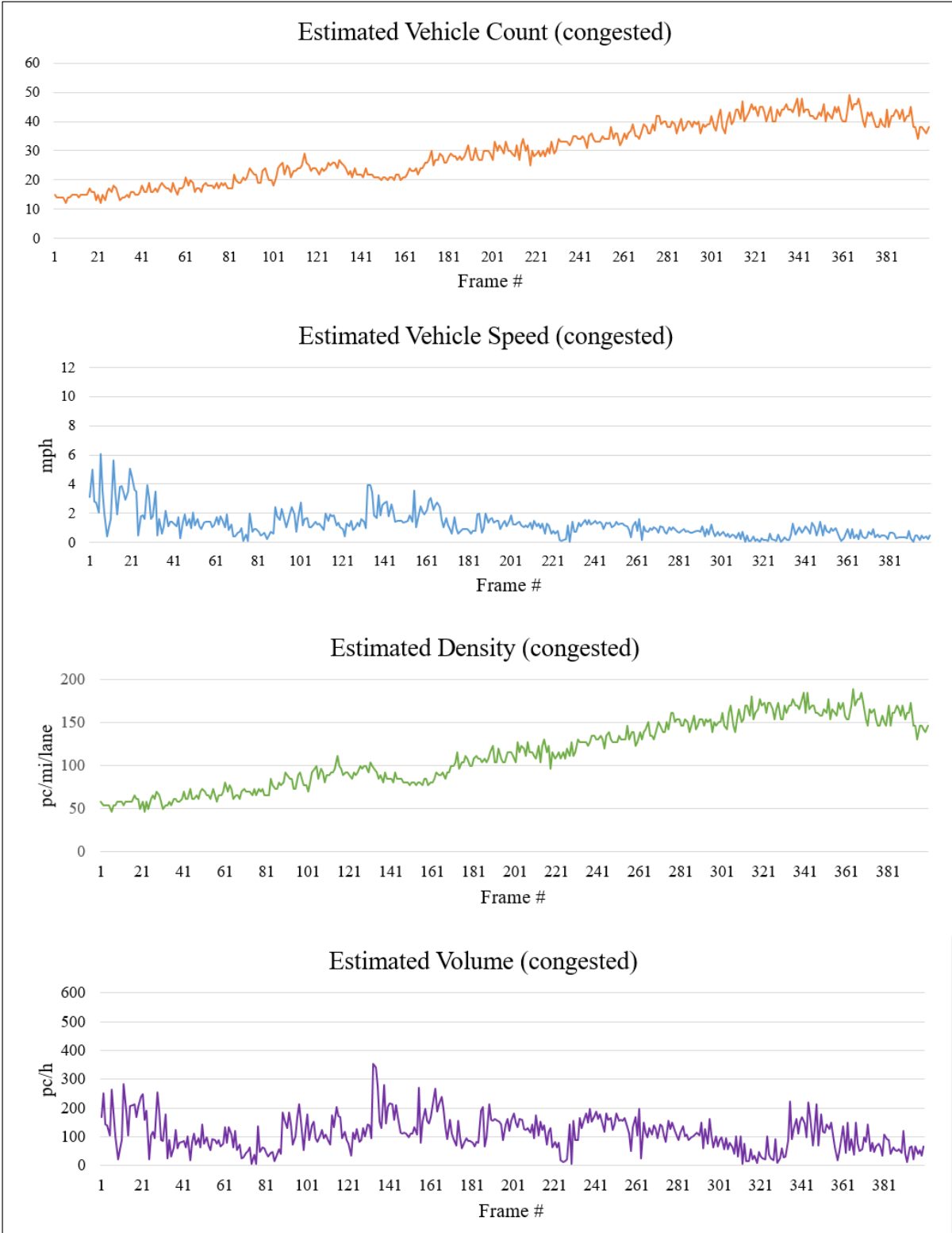
Figure 7-7 Estimated instantaneous traffic flow parameters for test video #8 with congested traffic
