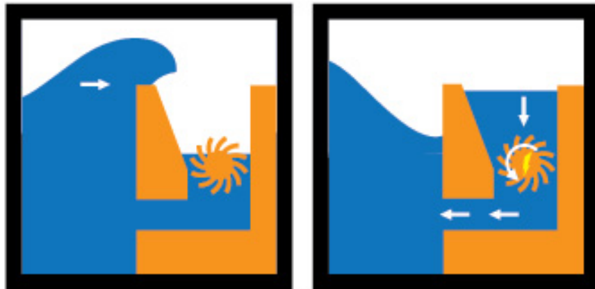
Figure 1.2: The main principle of an overtopping WEC is for the kinetic energy of waves to fill a reservoir with water. This potential energy buildup is converted to electrical power through a turbine at the reservoir outlet [19].
