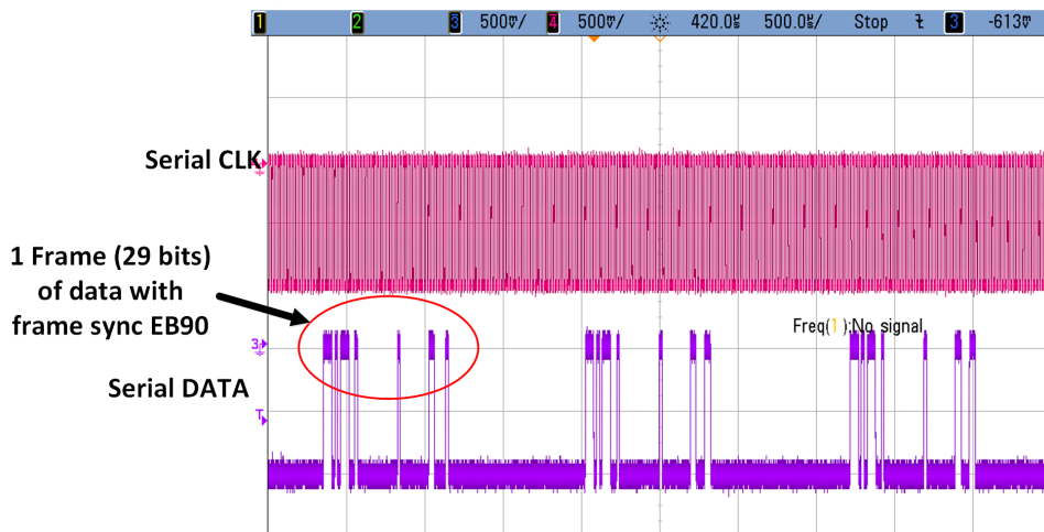
Figure 5.5: Serial output from the digital sensor interface
