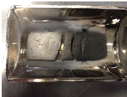
Figure 5.10 Image of 100% NH_3 600°C pyrolysis when the tube furnace had a measurable temperature variation.
