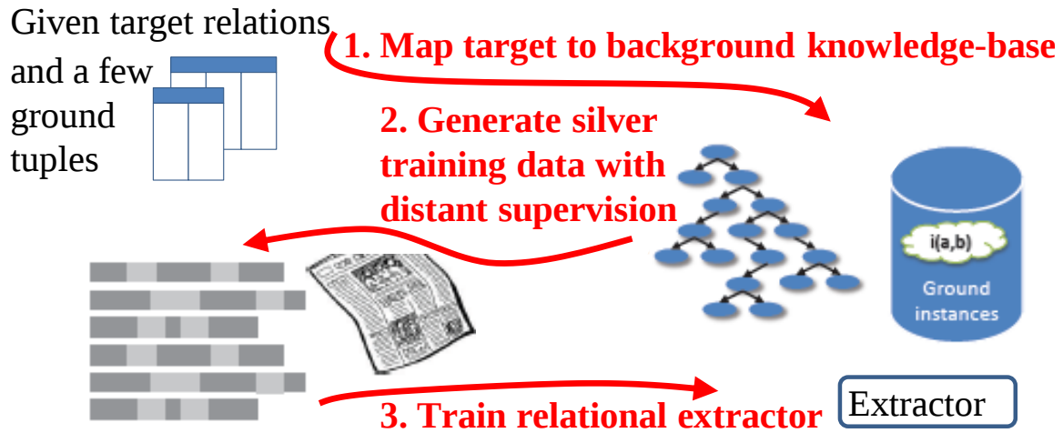
Figure 2.1: System overview of VELVET: first, it maps target relations to background knowledge based according to the given ground tuples; second, silver training data is generated with distant supervision; third, the relation extractor is learned from the silver training data.
