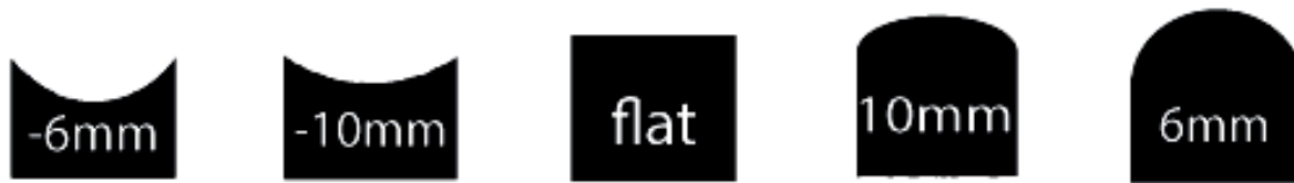
Fig. 2. From left to right, each radius of curvature from concave to convex is represented. These morphologies were modeled for final tooth plates.
