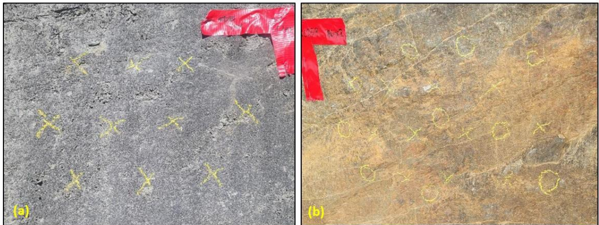
Figure 2.1 Examples of Schmidt hammer (SH) testing locations: (a) a grid set-up on the slope face (yellow X’s indicate impact locations) used for standard and “Super Sites” tested by one individual; (b) a grid set-up for two individuals taking measurements (indicated by yellow X’s and O’s).
