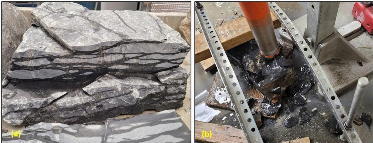
Figure 2.4 Examples of the LL71 mudstone behavior during sample preparation: (a) prominent bedding caused the rock to break apart into sheets of varying thickness; (b) an attempt to core a mudstone rock resulted in failure along the bedding and the disintegration of the sample.
