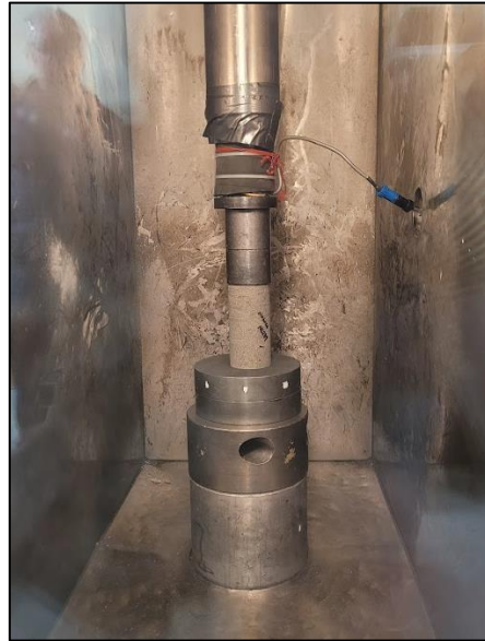
Figure 2.5 Cylindrical rock sample loaded into the UCS testing machine.
