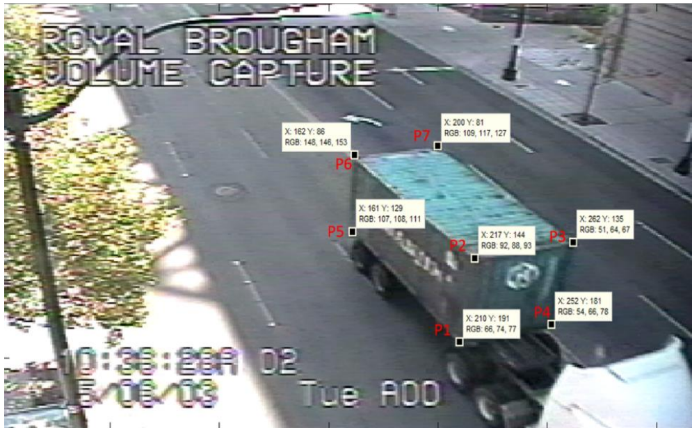
Figure 5-13 Identify the seven corner points and obtain their pixel coordinates for calibration.
