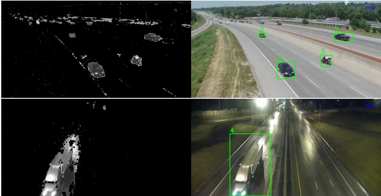
Figure 5-11 AI trigger method that uses traditional detection and tracking as the trigger, and the finetuned Mobilenet as the final classifier for traffic volume detection.
