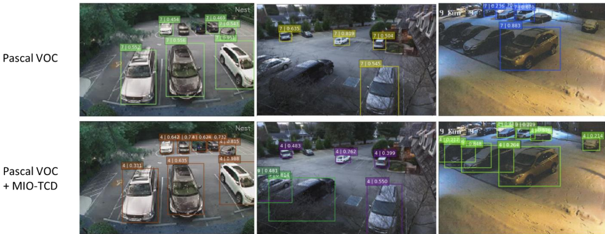
Figure 4-3 The enhanced SSD-Mobilenet Detector implemented at the edge of our system has a significantly improved detection performance, especially on challenging parking scenarios in surveillance image data.
