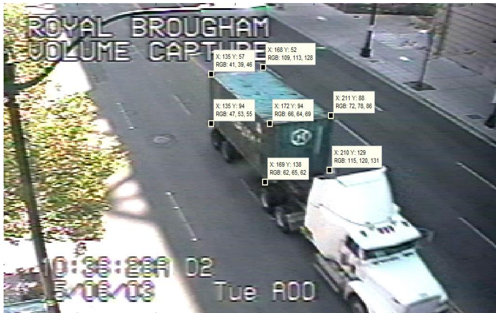
Figure 5-15 Verification using the pixel coordinates of the truck container in a different frame.
