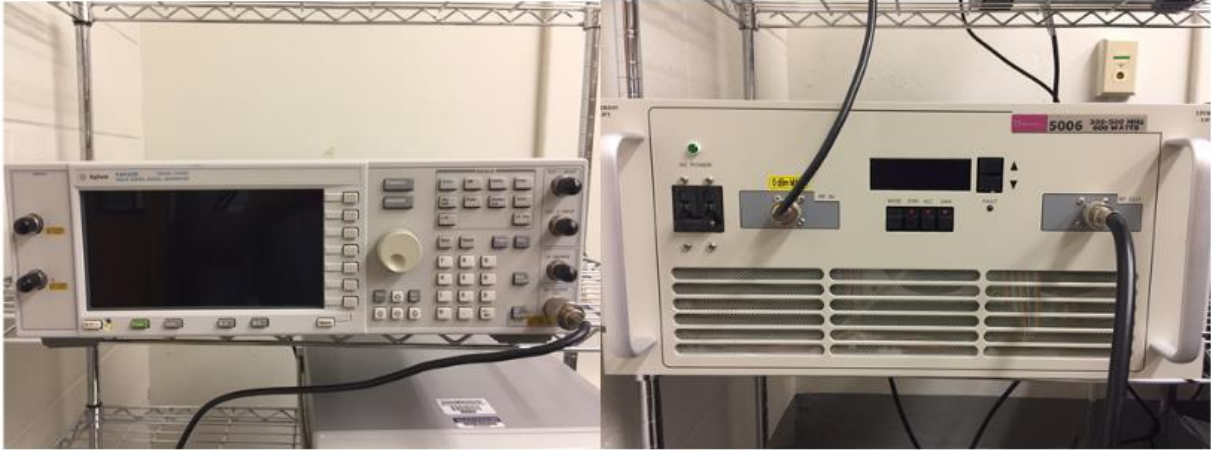
Figure 4-4 Left: signal generator. Right: power amplifier
