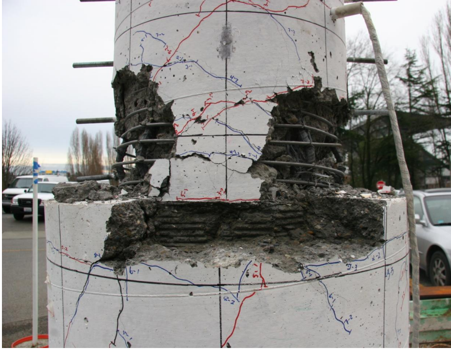
Figure 4-2. Specimen DS-1 after testing
