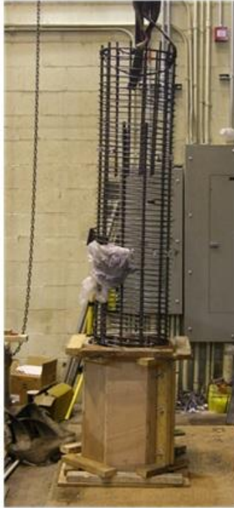
a). Column reinforcement
