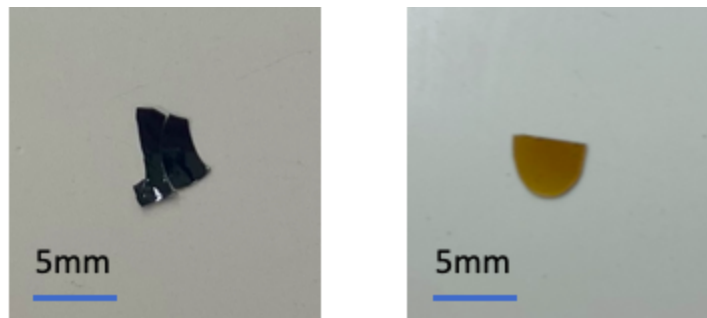
Fig 3.10. Intermediate products obtained from a separate run with step 1 only (RT - 350°C - 2h isothermal process). Left: in air. Right: in nitrogen.
