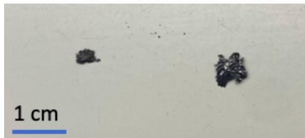
Fig 3.7. Final carbon products obtained from H_{300/900} . Left: without pre-pyrolysis oxidation (all processes were done in nitrogen). Right: with pre-pyrolysis oxidation.
