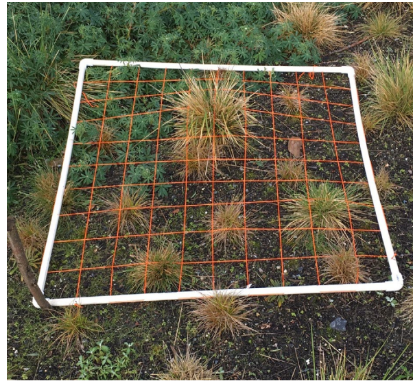
Figures 5.17 A 1x1 meter grid made of PVC pipe and string for grid sampling. Source: Jocine Velasco
