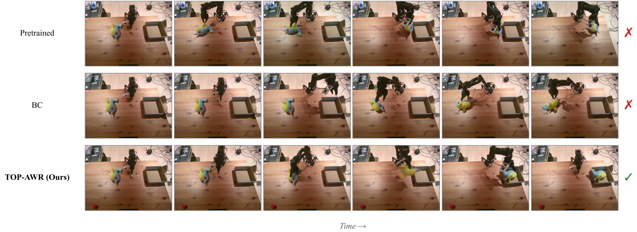
Figure B.8: Qualitative comparison on “Place doll in box.” The pretrained policy and behavior cloning (BC) both fail, while TOP-RWBC, fine-tuned with reward weights from TOPReward, succeeds consistently. Frames are uniformly sampled from evaluation rollouts.
