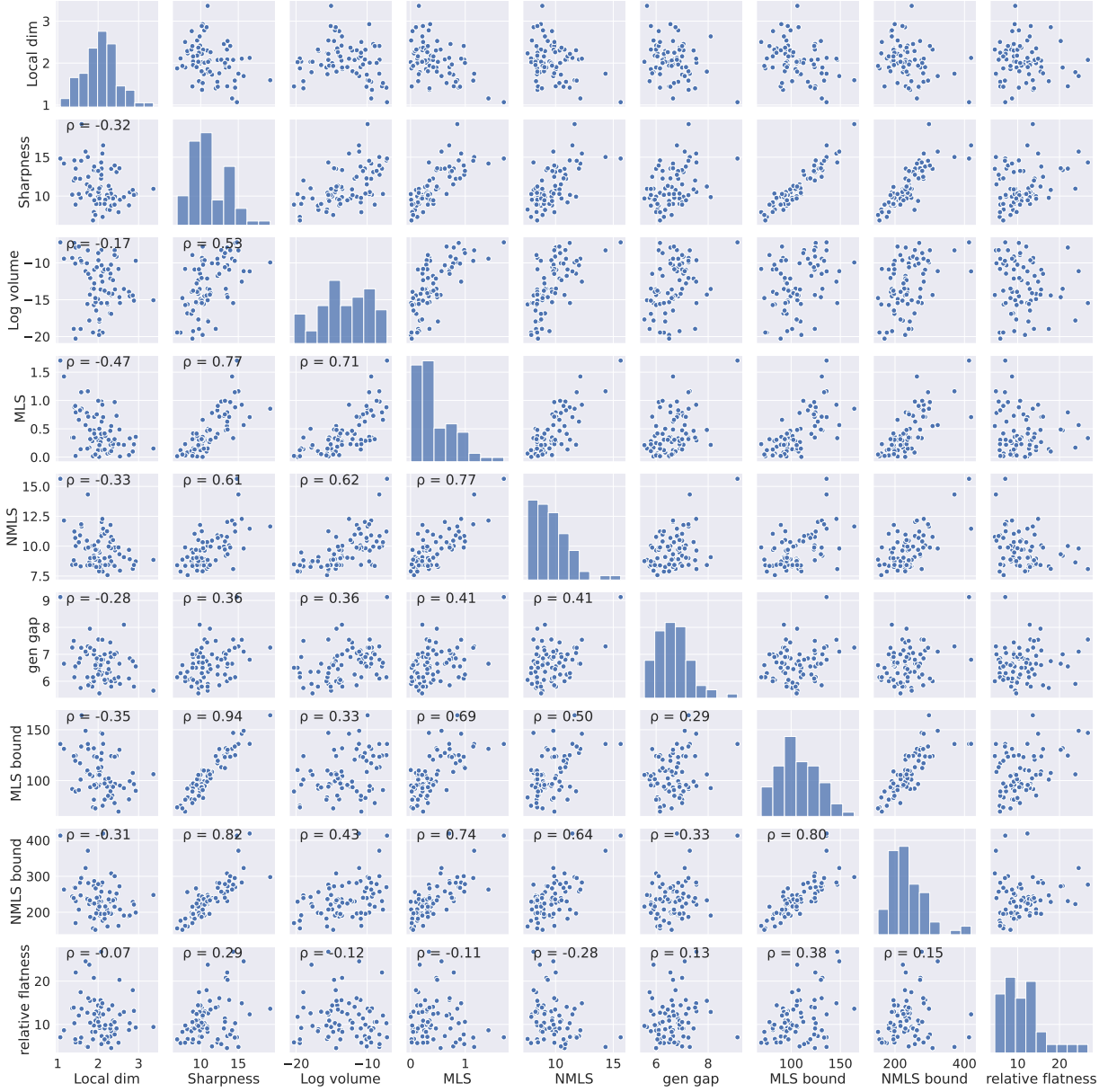
Figure D.8.4: Pairwise correlation among different metrics. We trained 100 different LeNets on the CIFAR-10 dataset using vanilla SGD with different learning rates, batch size, and random initializations and plot pairwise scatter plots between different quantities: local dimensionality, sharpness (square root of Equation (5.3)), log volume (Equation (5.7)), MLS (Equation (5.11)), NMLS (Equation (5.12)), generalization gap (gen gap), MLS bound (Proposition 5.8), NMLS bound (Proposition 5.10) and relative sharpness ([Petzka et al., 2021]). The Pearson correlation coefficient \rho is shown in the top-left corner for each pair of quantities. See Appendix D.8.2 for a summary of the findings in this figure.
