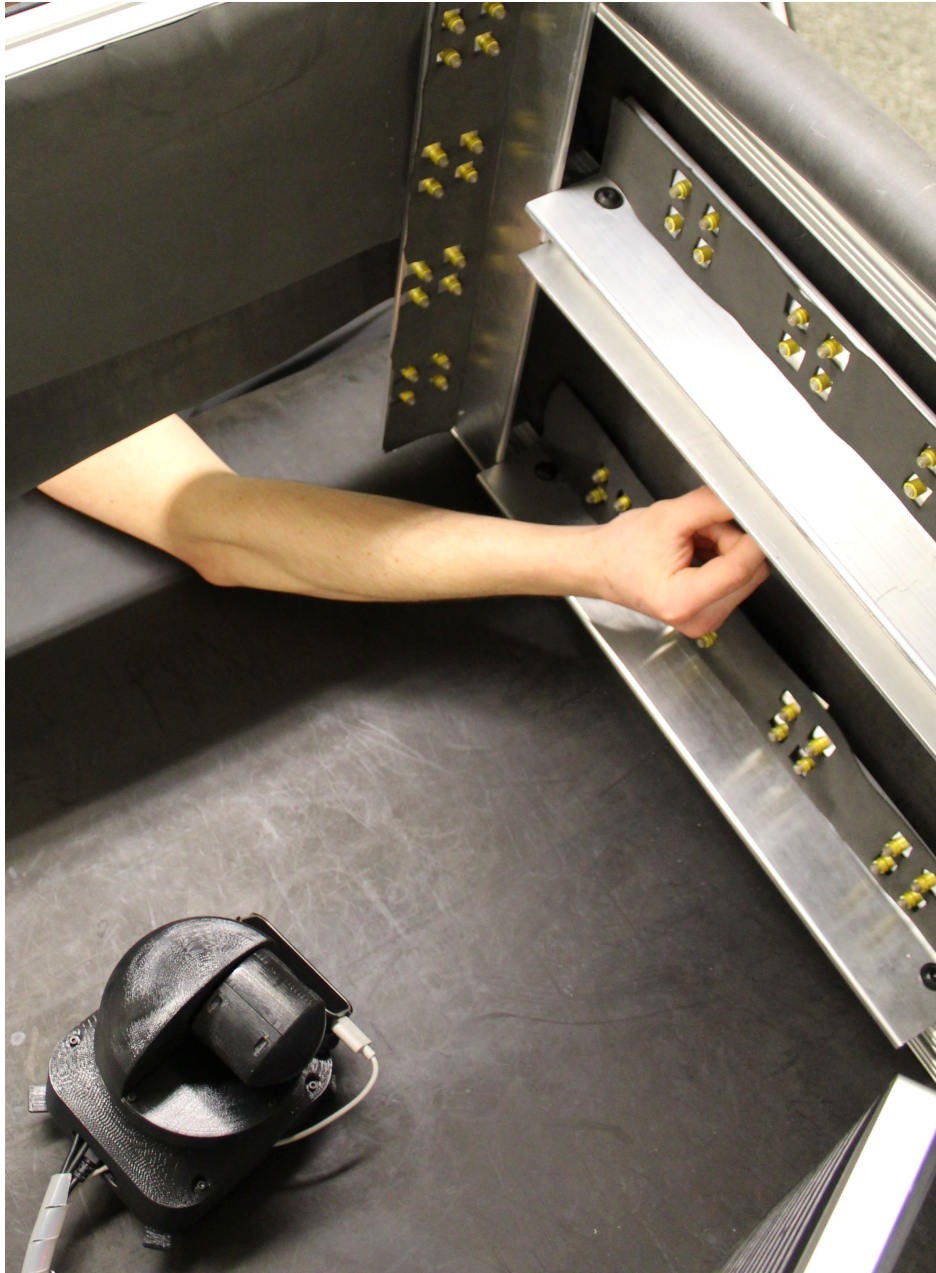
Figure 3.6: Experimental setup for inspection task with robotic assistant. Collars (yellow) are inspected for correct installation in their groupings of four.
