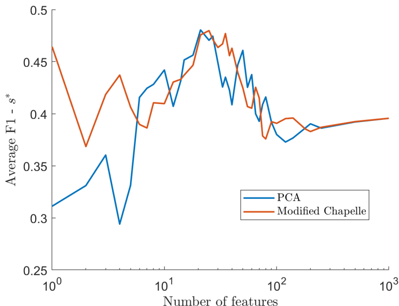
Figure 5.6: Recursive feature selection performance results for the online classification task, measured in average F1 measure across all ten subjects. Performance at the 99.9% accuracy retention cutoff established in Table 5.1 is near a peak of 15% better F1 performance relative to the full-featured data, indicating that problematic features have been removed effectively. Additionally, in the extreme case of using only a single feature out of 4551 total there is a 49% performance improvement if that feature is selected by the modified Chapelle method rather than by PCA.
