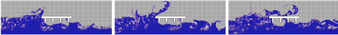
Figure 3.5: Time-lapsed figures (from left to right) of flow mixing and wave breaking near the bridge superstructure during impact in the two-dimensional laminar flow case.
