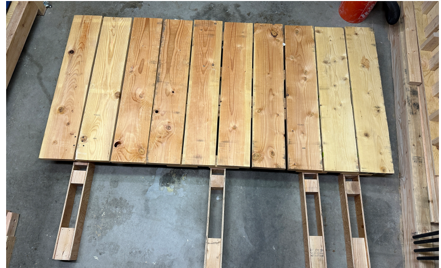
Fig. 68 Platform w/ base assemblies for FFS
