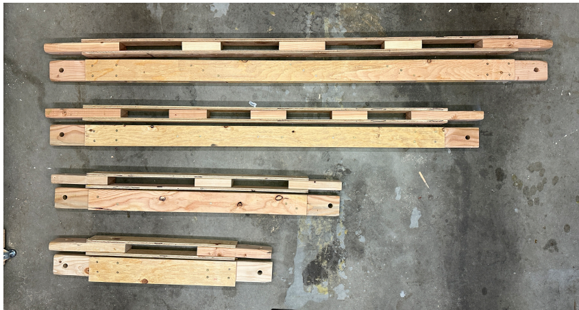
Fig. 66 Flexible Framing System (FFS) components clockwise from top right: mortise and tenon joint w/dowel, Base frames w/mortise in the center, Horizontal assemblies at different lengths, tools for assembly: Tape measure, mallet, dowel
