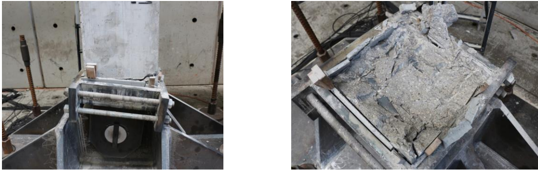
Figure 5.24: Base of the Column After Out-of-Plane Failure Occurred
