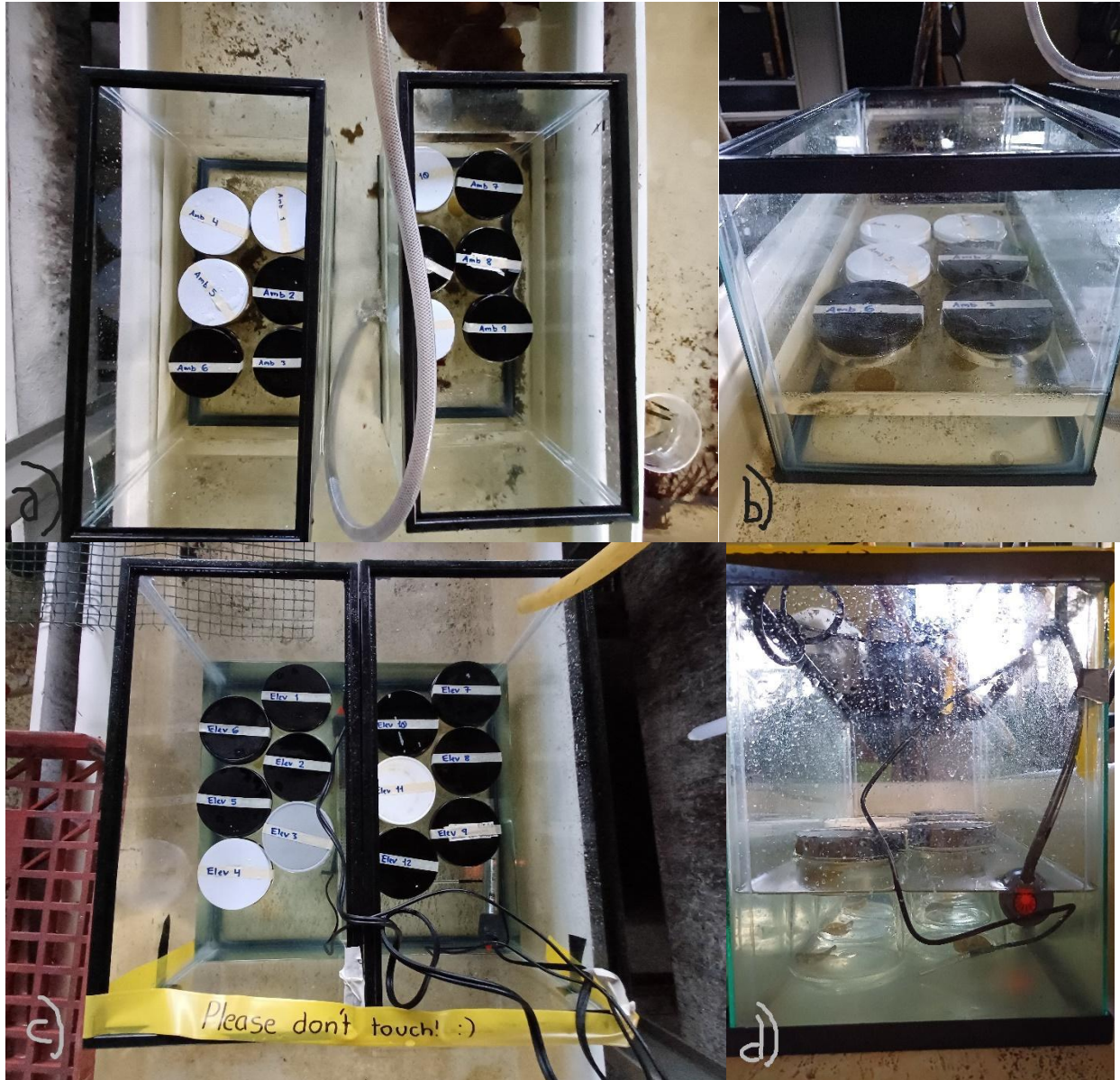
Figure 3. Ambient (a,b) and elevated (c,d) temperature treatment setups. a) Overhead view of two ambient temperature aquarium tanks in a sea table with flowing seawater from the Puget Sound. b) Side view of an ambient temperature aquarium tank. Note that one kelp disc is present in each of the 6 mason jars in the tank and that the water level of the sea table is equal to that inside the aquarium tank. c) Overhead view of two elevated temperature aquarium tanks in an empty sea table. d) Side view of an elevated temperature aquarium tank. Note that one kelp disc is present in each of the 6 mason jars in the tank and an aquarium heater is present to heat the tank to 18 °C.
