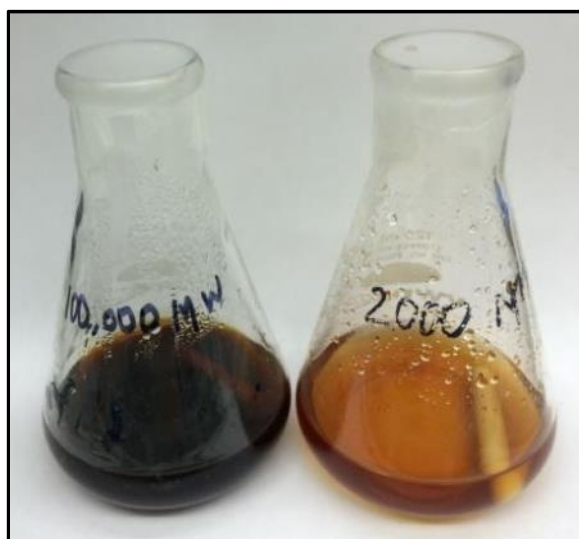
Figure 2.3.6: Synthesis of silver nanoparticles with 100K MW (left) and 2K MW (right) PAA
