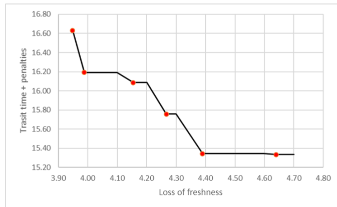
Figure 4.1: Comparison of objective functions on the baseline expected value test problem. The line represents the efficient frontier of the Pareto analysis and the red dots denote calculated solutions that are non-dominated.
