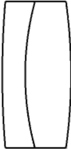
Figure 1.5 A lens diagram of an achromatic doublet.
