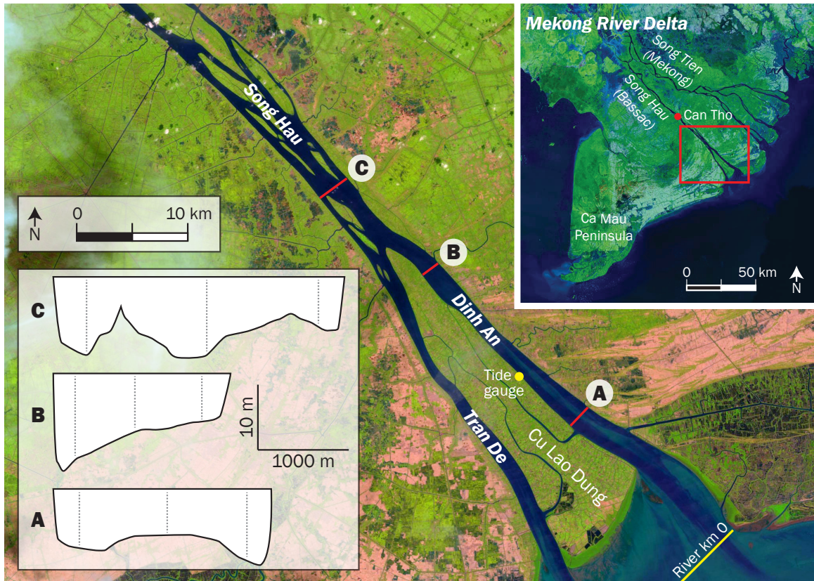
Figure 4.1: Study area basemap with Landsat 7 ETM imagery acquired 13 February 2002. Map at top right shows greater Mekong River Delta region. Red lines denote cross-sections occupied during the two cruises. Inset at lower left shows generalized bathymetry as viewed downstream, with nominal station locations indicated by dashed vertical lines. The mouth (river km 0) is defined as the cross-channel extension of the left-bank limit. This is seaward of Cu Lao Dung's subaerial extent but representative of the geomorphic transition from river to open ocean given the extensive flats fronting Cu Lao Dung.
