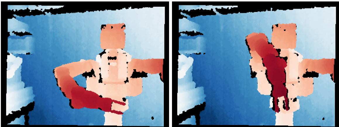
Figure 3.1: An example scenario showing the initial (left) and target depth clouds (right). SE3-POSE-NETS can be used to control the robot to reach the target state based on raw depth (and optionally, color) data. Depth images colorized for display purposes only.
