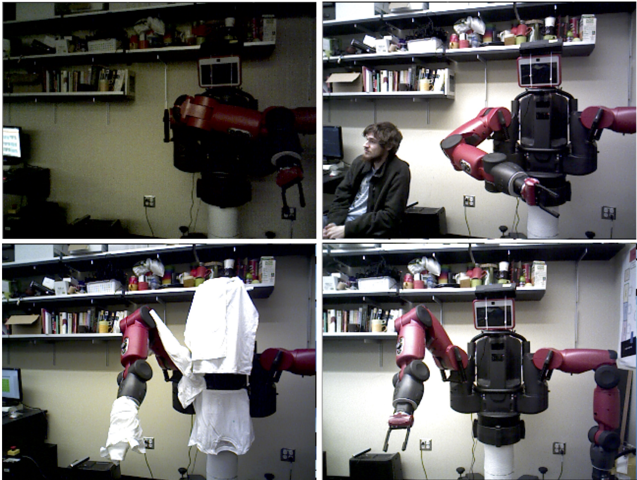
Figure 3.9: Examples of different generalization tests, unseen during training. Clockwise from top left: 1) Low light setting, 2) Motion in the background (person on the chair moves), 3) Fixed distractor(s) in the foreground (white towels on the robot) and 4) Change in camera pose (rotated \sim 10 degrees to the right). SE3-POSE-NETS are robust to these changes, achieving good control performance on a majority of our tests with these perturbations.
