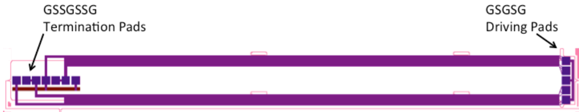
Figure 8. Termination pad configuration for the Mach-Zehnder Modulator
