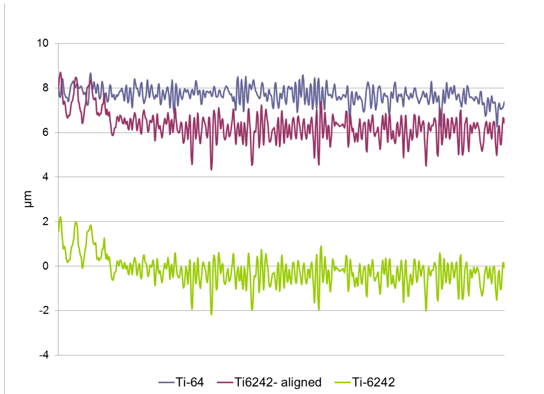
Figure 5.2-2: Surface Profiles of Dissimilar Ti-Alloys Aligned for surface characteristics at Bonding Interface
