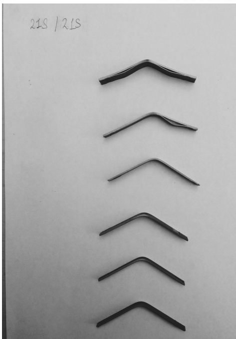
Figure 4.2-37: Fractured Specimens from lower to higher temperatures in DB Similar \beta Ti-Alloys ( \beta -21S/ \beta -21S)
