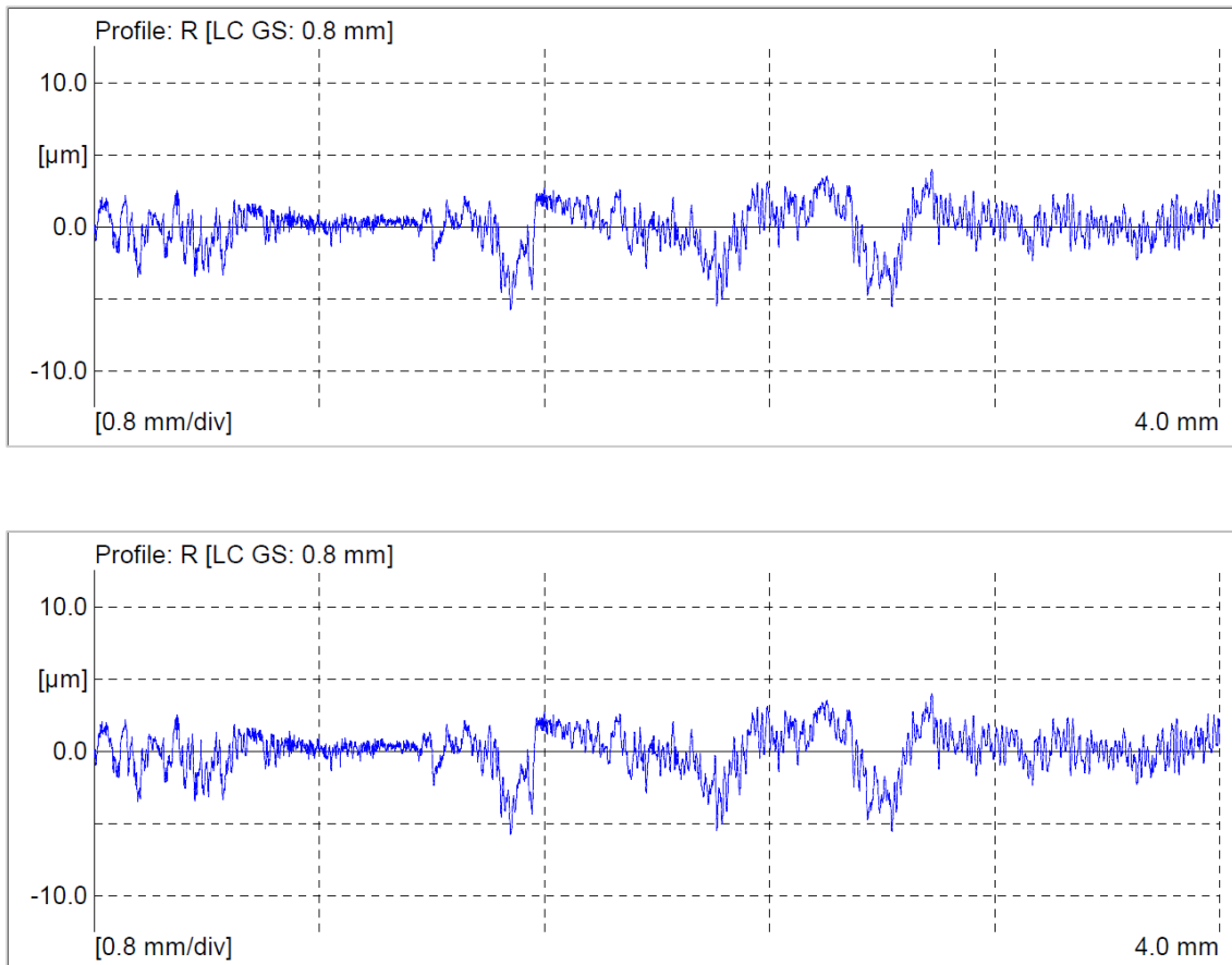
Figure 5.2-1: Typical Surface Profile of Parent Alloys –Ti-64SG/Ti-6242SG
