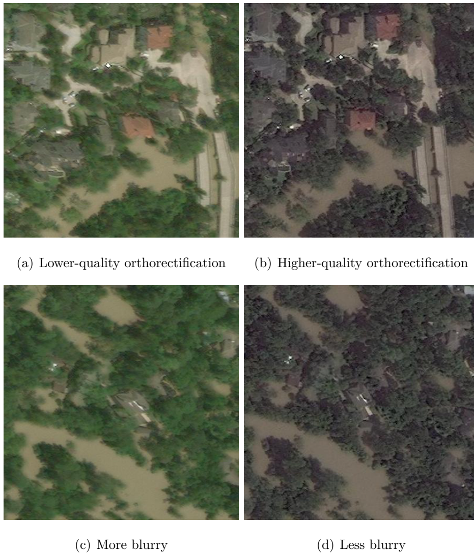
Figure 2.3: Different orthorectification and pre-processing quality of the same location on different days.
