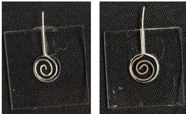
Figure 5.2. Picture of silver wire electrode (left) and synthesized silver chloride electrode (right).
