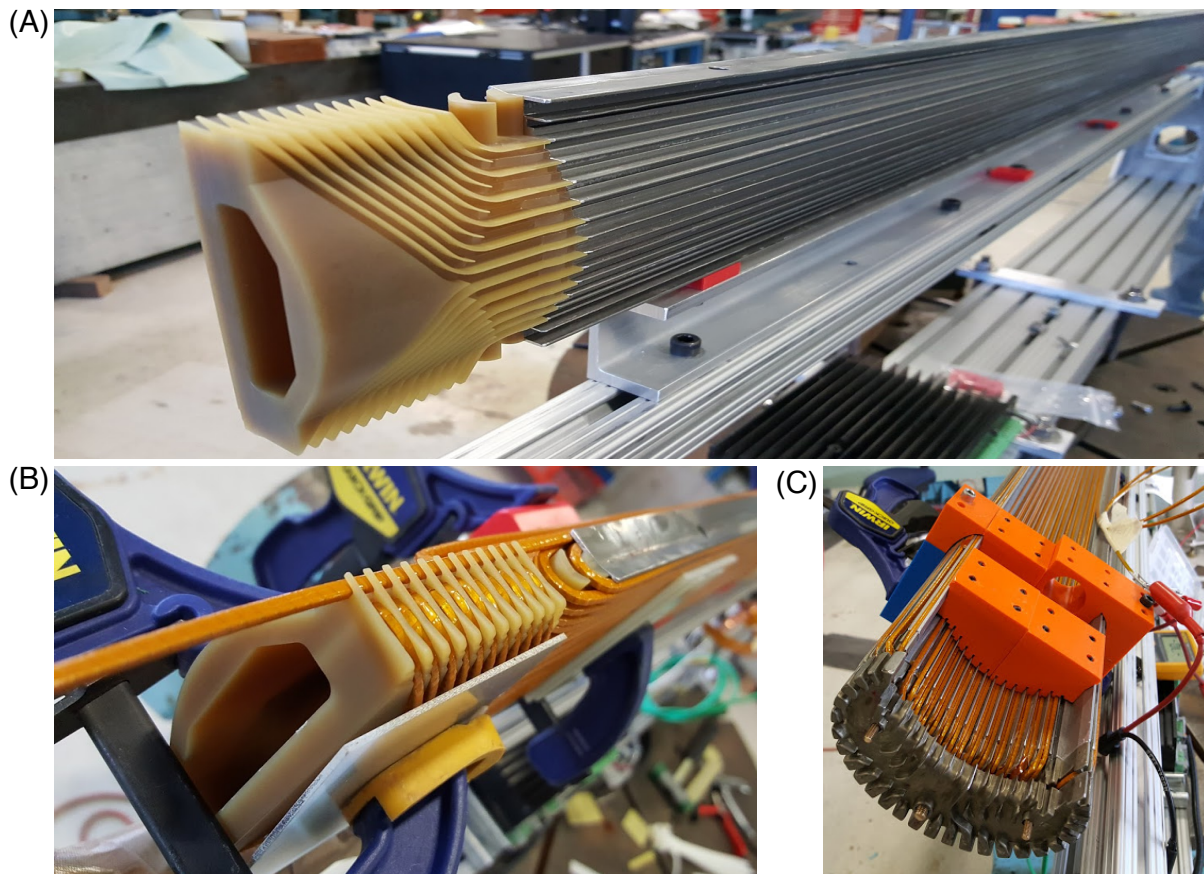
Figure 3.34: (A) Upstream end of inner coil mandrel with redesigned end. (B) Wrapped inner coil, downstream end. (C) First layer of wrapping of the outer coil, with jig for testing electrical shorts to the body of the aluminum mandrel.
