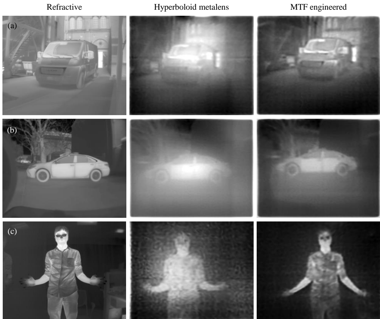
Figure 5.4: LWIR imaging “in the wild”. Three scenes were imaged using the refractive LWIR lens (left), the hyperboloid metalens (middle), and the MTF engineered meta-optic with complex scatterers (right). Scenes (a) and (b) were captured outdoors on a sunny day while (c) was captured indoors.
