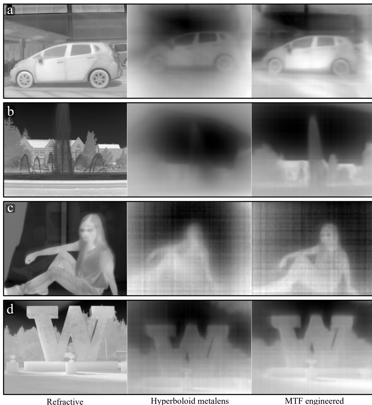
Figure 5.9: LWIR imaging “in the wild”. Four scenes are imaged using the refractive LWIR lens (left), the hyperboloid metalens (middle), and the MTF engineered meta-optic with complex scatterers (right). The four scenes were all captured during daytime on a sunny day depicting (a) a parked car on a sunny day; (b) a fountain in the foreground against a building in the background; (c) a woman resting against a window; (d) a metallic structure.
