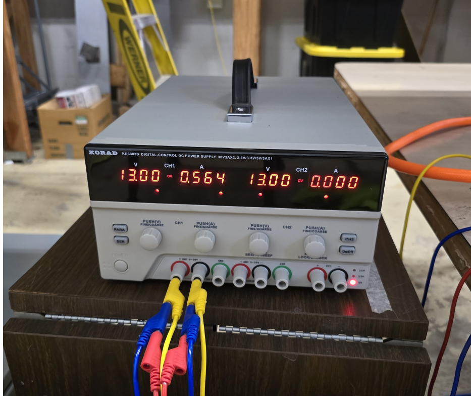
Figure 3.17: Power supply used to actuate the pneumatic solenoid valves.
