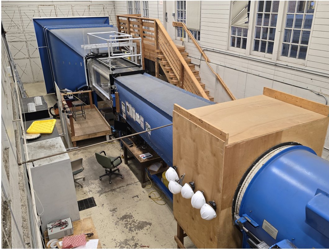
Figure 3.1: University of Washington AERL 3 ft \times 3 ft low-speed wind tunnel.
