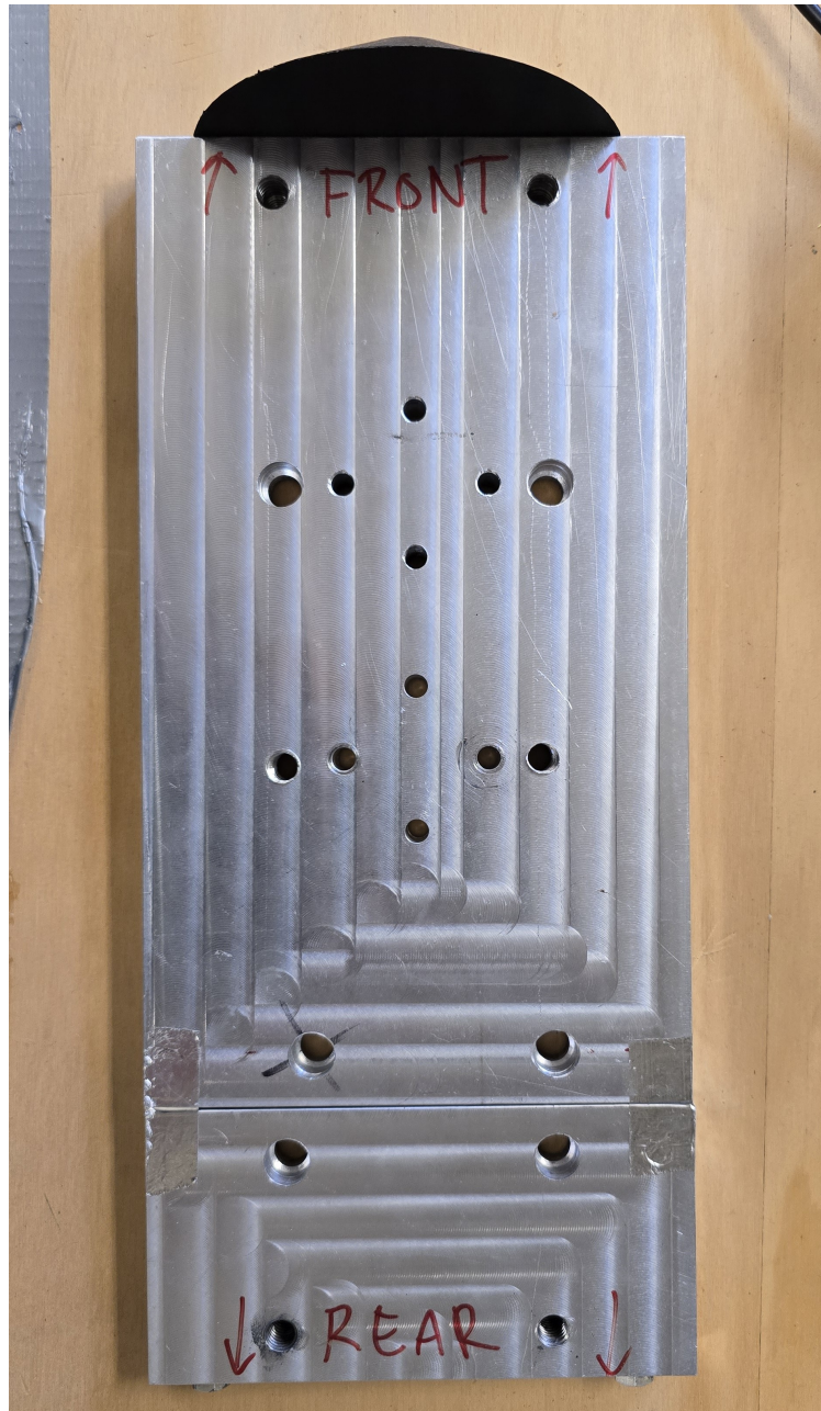
Figure 3.3: Custom-machined aluminum mount plate used to interface the wing model with the half-body force balance [33].
