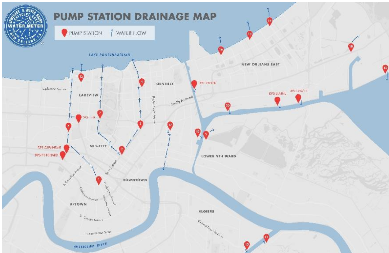
Figure IV-J SWBNO Pump Station Drainage Map
