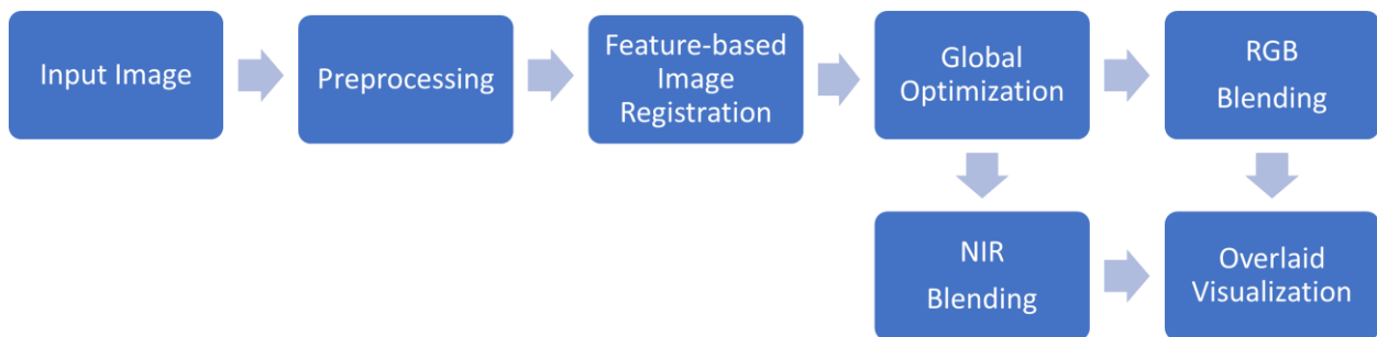
Figure 6.5 Pipeline for 3D multimodal esophagus reconstruction
