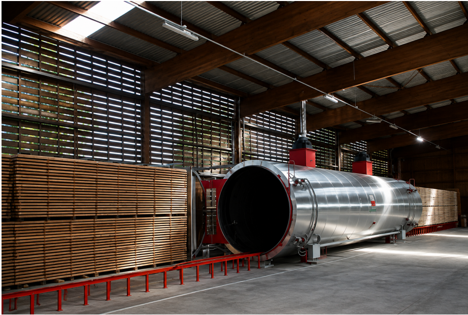
Figure 2.3: Maspell Thermo-Vacuum system at CRTC used for thermal modification of Western Hemlock boards
