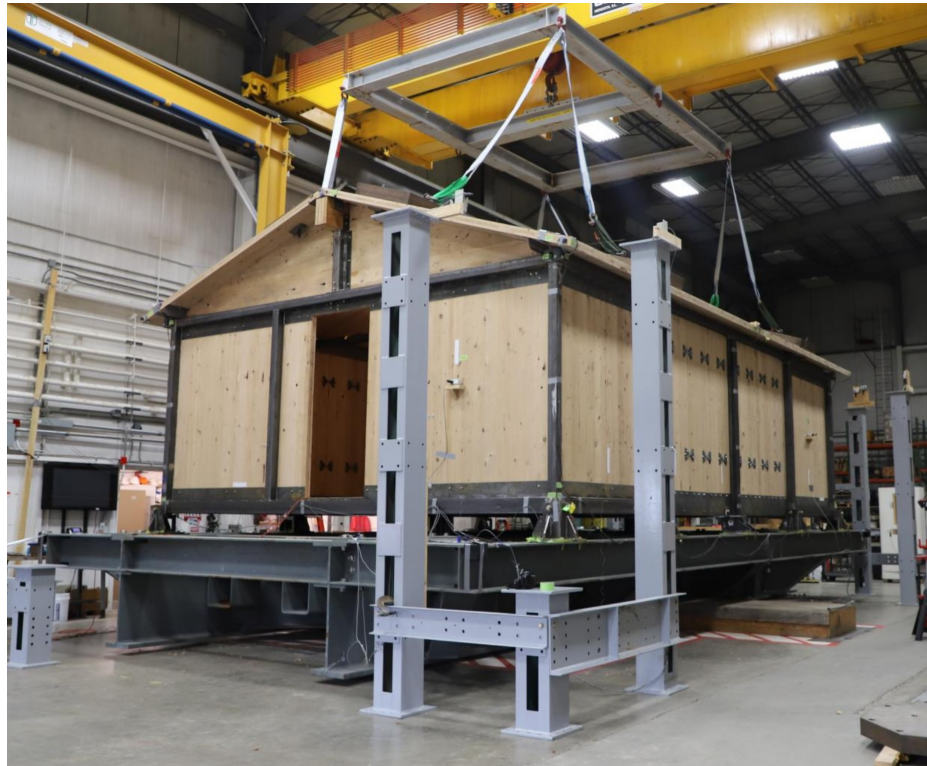
Figure 1.12: Full-scale seismic testing of a timber-based military shelter conducted as part of the U.S. Army ACLT Project
