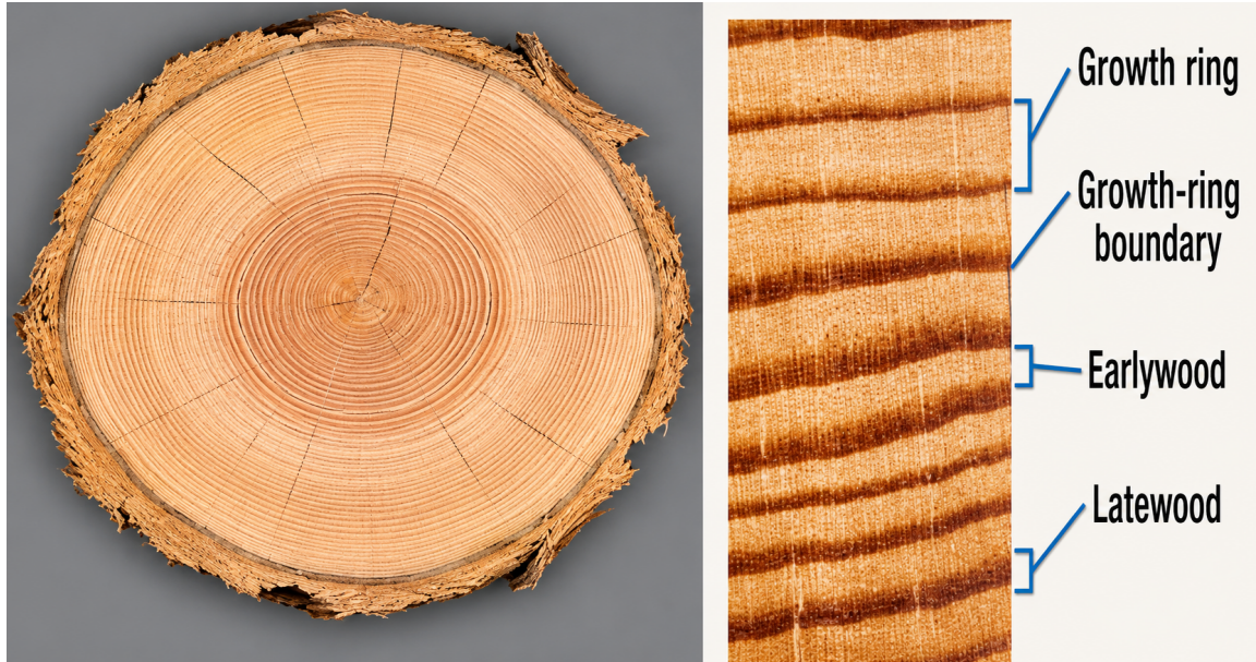
Figure 1.5: Macroscopic structure of wood showing growth rings, growth-ring boundaries, earlywood, and latewood.
