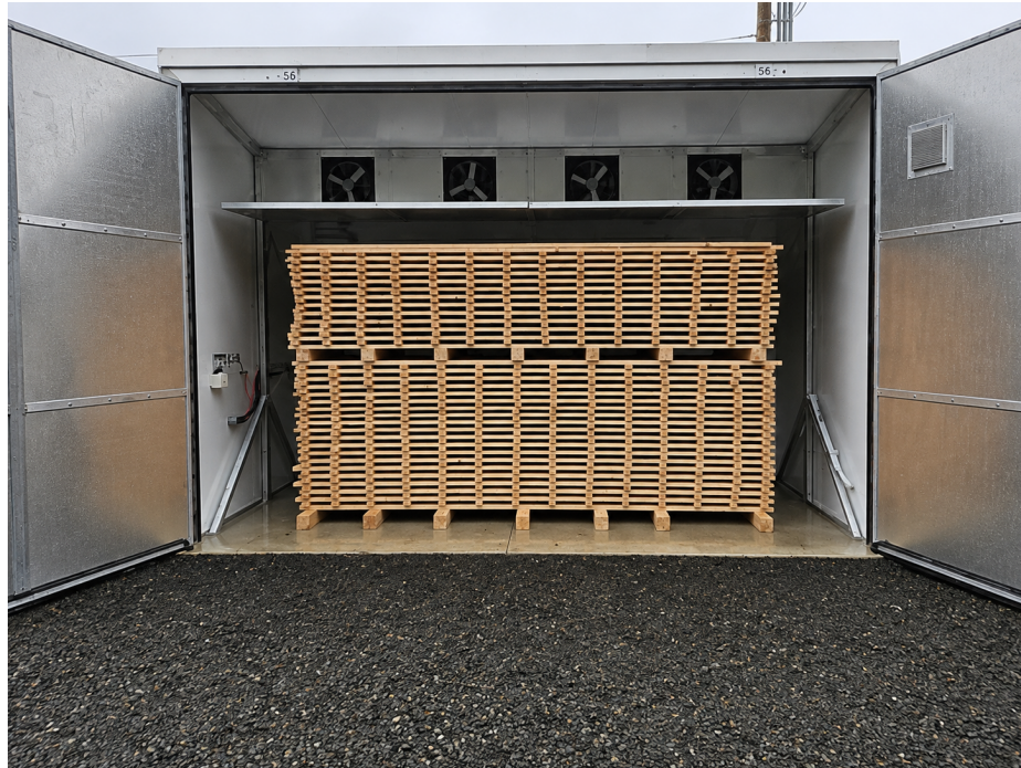
Figure 2.2: Kiln drying of Western Hemlock boards at Makah Sawmill
