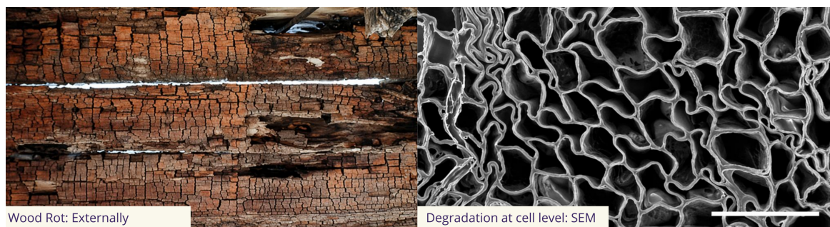
Figure 1.11: Moisture-induced degradation of wood at the macroscopic and cellular scales [4]
