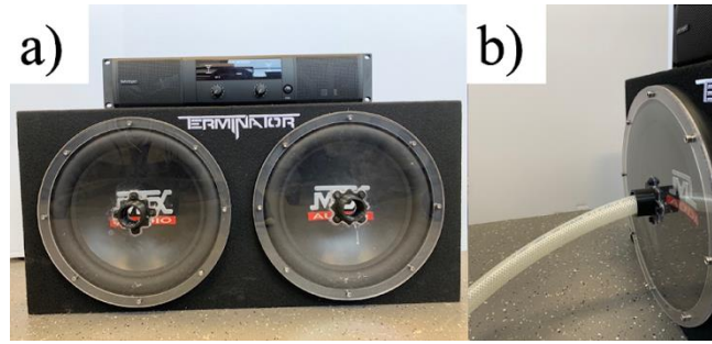
Figure 3.3.1. a) 3000W Class-D Amplifier on top of the modified subwoofer, and b) high air pressure tubing carrying air pressure waves from the modified subwoofer cone encased in acrylic.
