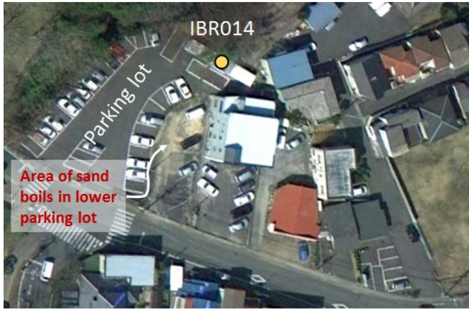
Figure 7.10: Aerial photo showing the location of ejecta after Tohoku earthquake. Aerial photo of the site taken on March 28, 2011, showing the extent of ejecta in the lower parking lot. Image courtesy of Google Earth, GeoEye.
