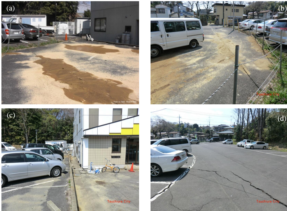
Figure 7.9: Photos showing surficial evidence of liquefaction at IBR014. (a) Ejecta in the lower parking lot shortly after the Tohoku earthquake. Image courtesy of Yoshiya Hata. (b) Photograph of surface ejecta in the lower parking lot. (c) Photograph of minor retaining wall failure. (d) Photograph of cracks without ejecta in the upper parking lot. Images courtesy of Jon Stewart, GEER taken on March 31, 2011.
