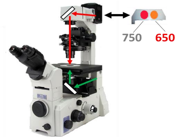
Fig. 4.21 Microscope set up for TIRF imaging and opto-PI3K.
