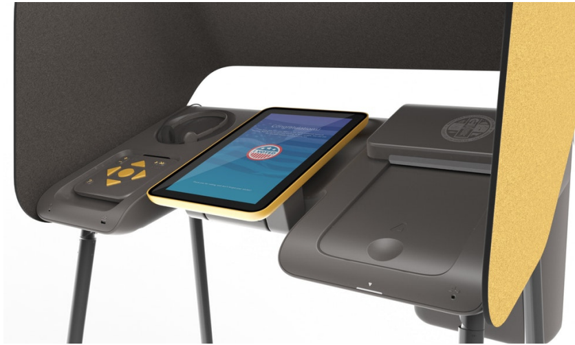
Figure 3.3: A computer-rendered image of the final design for the voting machine, showing the machine’s digital and tactile interface.
