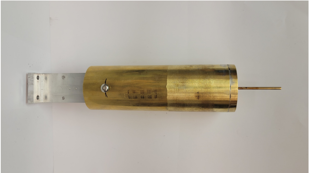
Figure 4.4: The assembled modified FIG diagnostic. The FIG is sheathed inside the large brass with a pitot-end on the right and a sealed end with a small opening for the connector cable.
