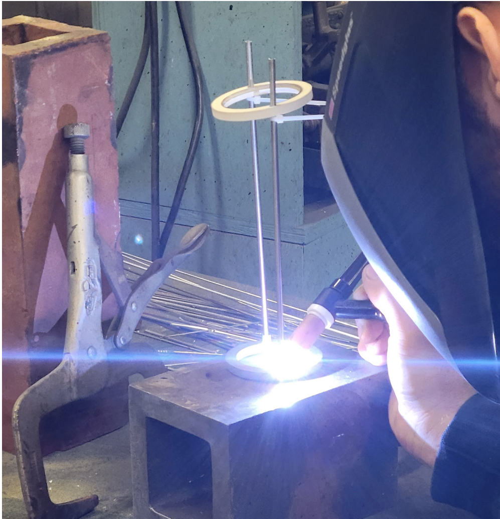
Figure 3.13: Welding steel gas tubes to the rear inlets of the 3D- printed anodes. The ACME ceramic anode insulator is used as a jig for correctly positioning the tubing. This welding was the only additional manufacturing step conducted after receiving the printed anode bodies of A3 and A4.
