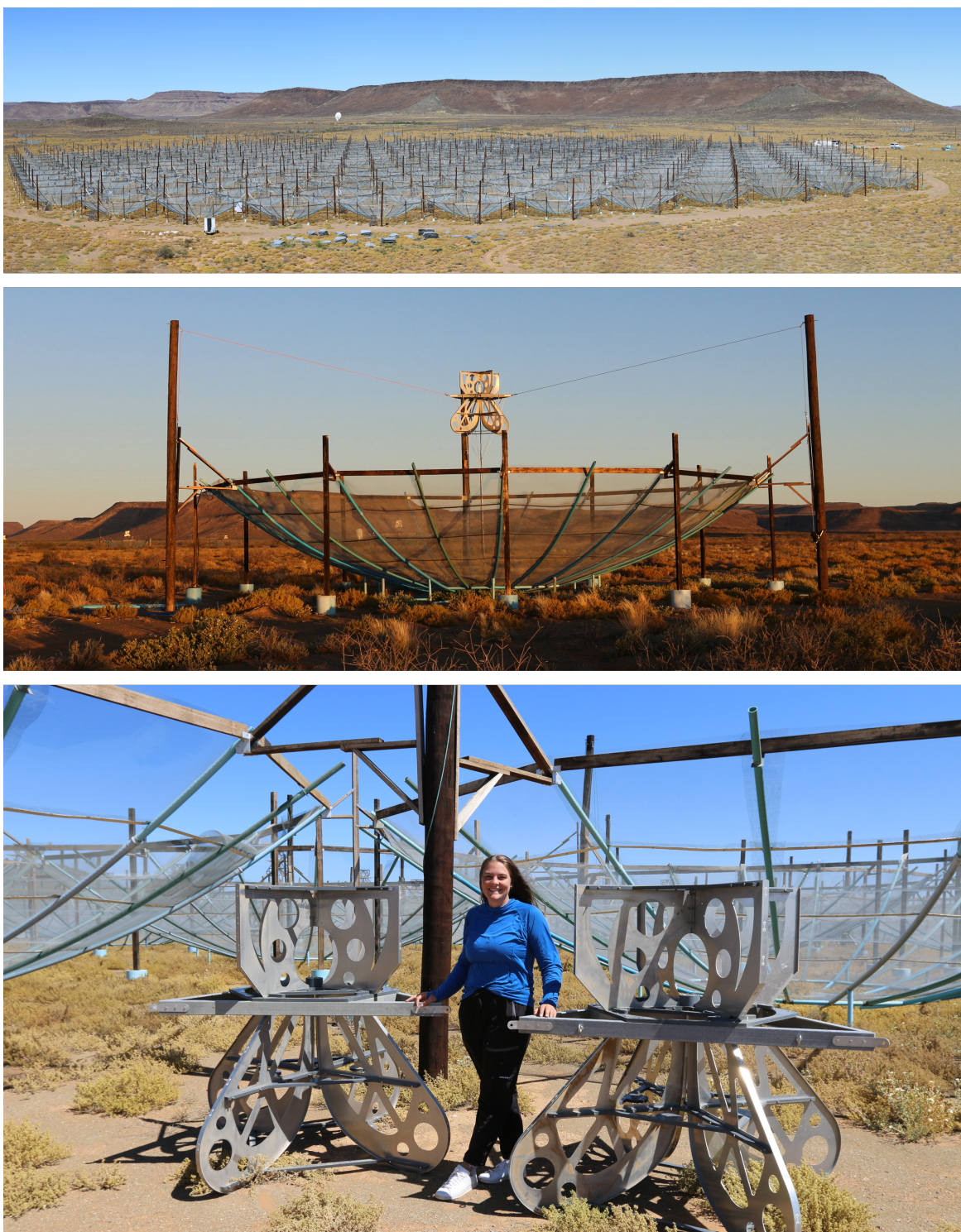
Figure 1.4: HERA's compact core (top), outrigger antenna (middle) and Phase II Vivaldi feed (bottom).
