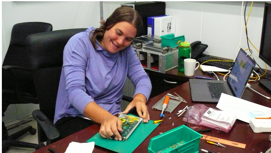
Figure 4.10: Picture of myself in the HERA onsite lab sliding a refitted PAM with conductive foam back into its housing. As part of the refit we removed as much dust and sand from both the boards and the housing as possible, but nonetheless grit on the rails made it quite strenuous to both remove and replace the PAM boards. This is evidenced by both my facial expression and my Band-Aid.
