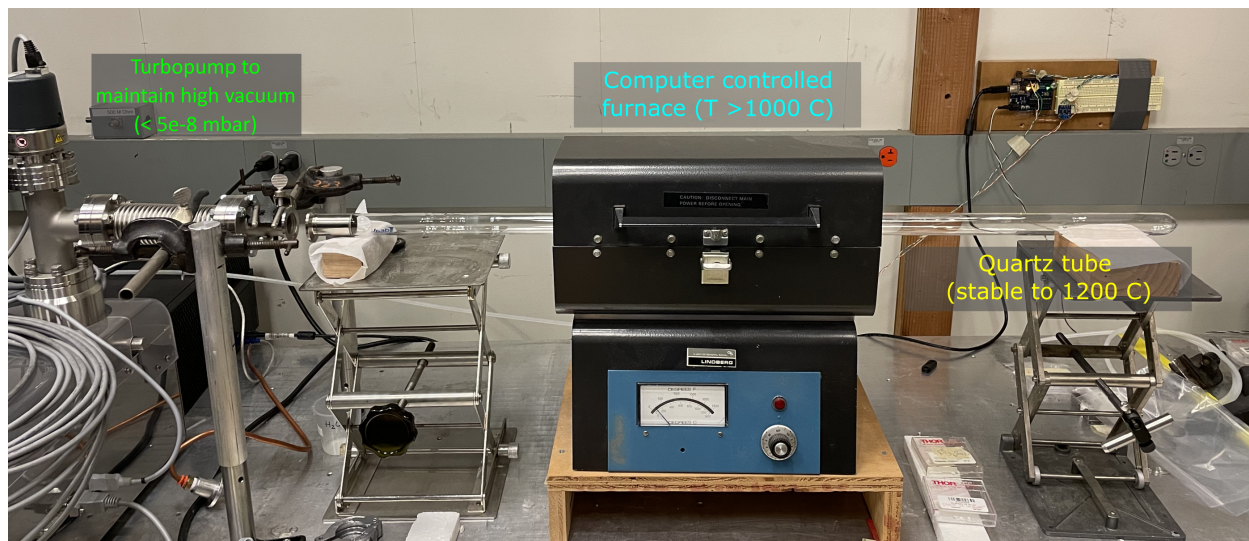
Figure F.1: The vacuum annealing setup consisting of a turbo pump directly connected to a single ended quartz tube (via KF-25 vacuum fitting). The quartz tube sits inside a tube furnace that is controlled by a computer interface.
