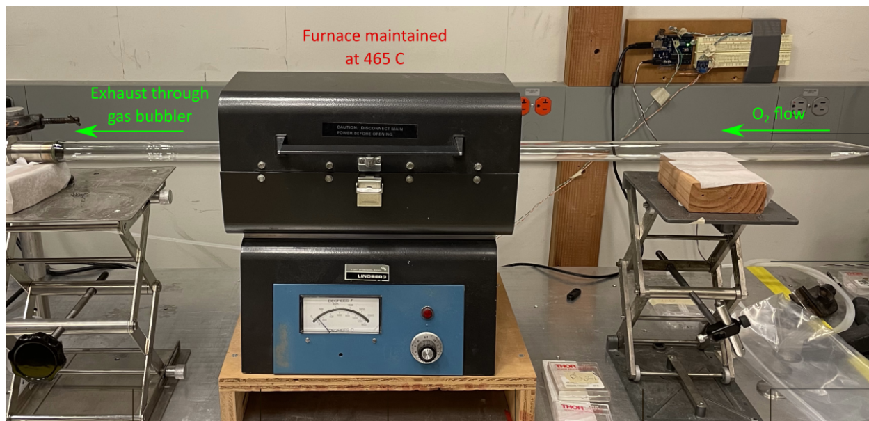
Figure F.3: The oxygen annealing setup consisting of a double ended quartz tube. One end is connected to the oxygen gas supply, whereas the other end is connected to a gas bubbler.
