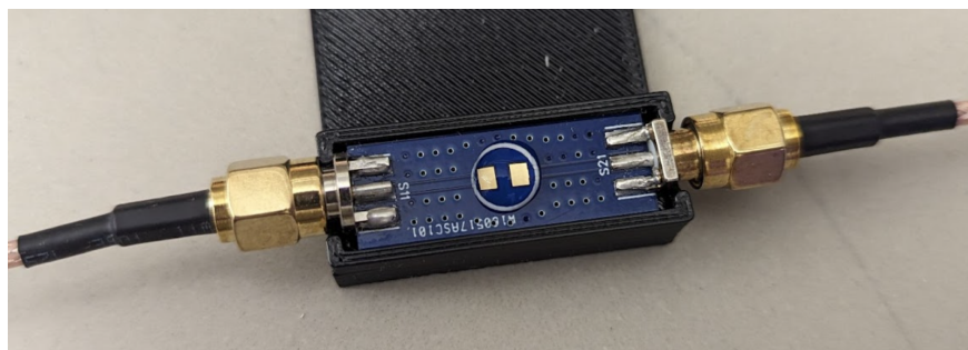
Figure 6.1: The board we designed leaves the circuit open until liquid solution (about 30 L) is placed in the circle. At that point, the signals generated by the VNA run through the solution and the response is measured on the S11 and S21 ports.
