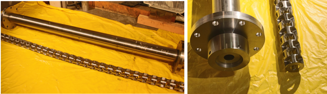
Figure 3.9: 2-meter section with associated flanges, end caps, and baffled inserts; end view of 2-meter tube with finned projectile for reference.
