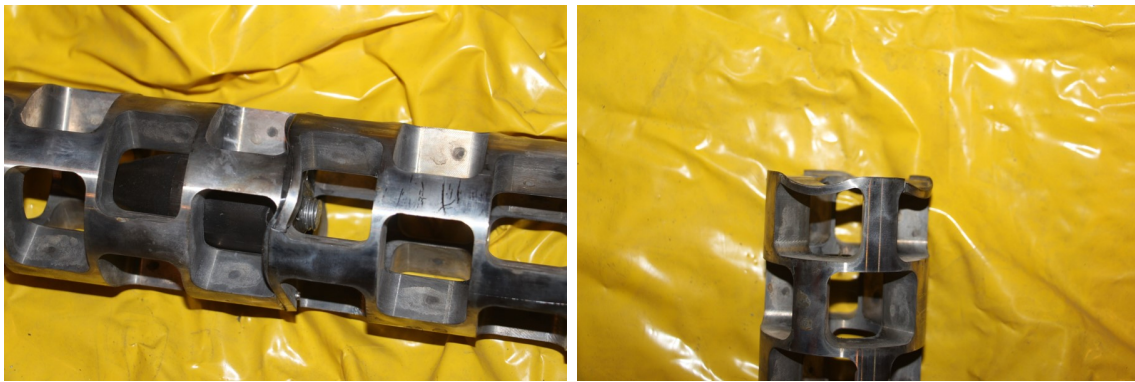
(a) Yielded inserts with localized failure; projectile broken in half and stuck. (b) Failed baffled at downstream end.
