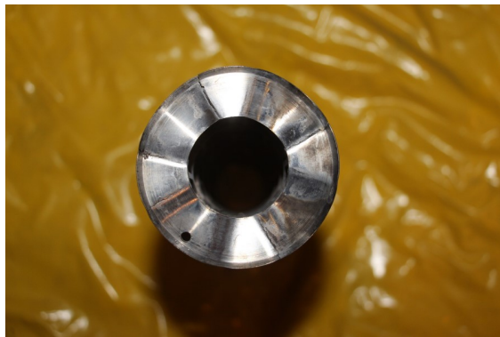
(c) Head on view of failed insert showing failure points, comparable to FEA model.
