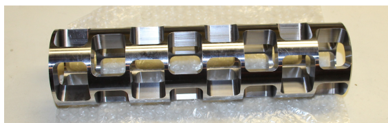
(a) Manufactured baffled-tube insert.
