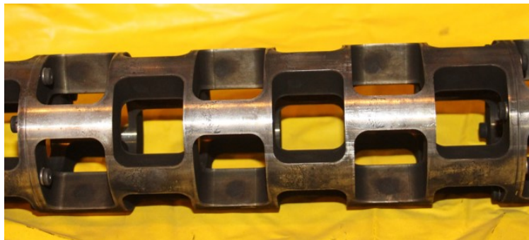
Figure 5.8: Combustion pattern on the baffled-tube inserts' rails.
