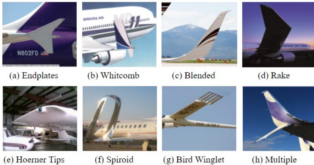
Figure 2-84 Configurations of various wingtip devices [89][90][91].
