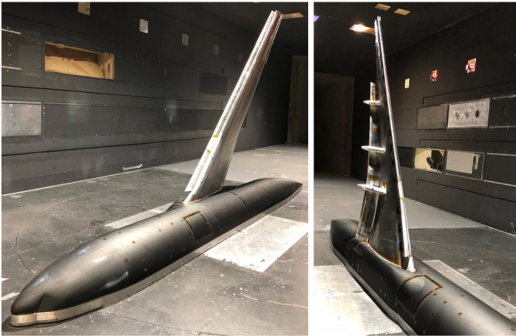
Figure 1-3 Components and actual photographs of the NASA HL-CRM at NASA Langley Research Center [23][28].
