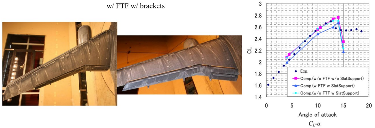
Figure 2-6 Measured surface flow pattern and comparison of aerodynamic forces [43].
