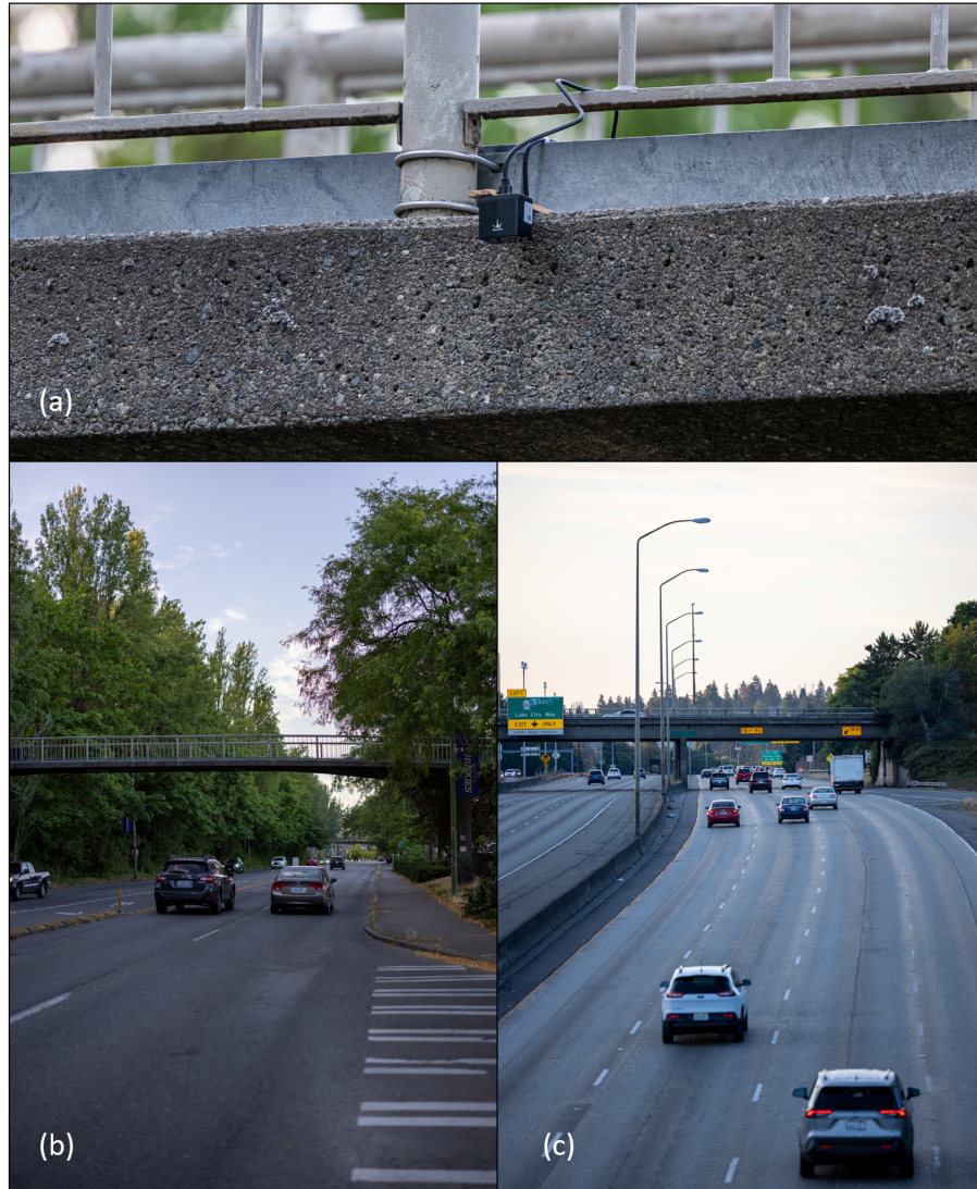
Figure 8.8: The data collection illustration. (a) visualize the installation angle of CLEVER compact LiDAR for vehicle represent sequence collection. (b) and (c) are the two overpasses used for data collection, both located in the city of Seattle, Washington State, USA.
