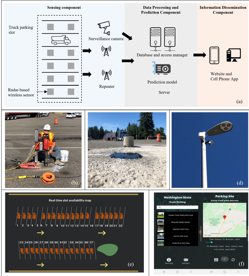
Figure 5.12: The architecture of the smart parking information management and prediction system in the pilot test bed. (a) the overall structure of the SPIMP used in the pilot project, including sensing, data processing and prediction, and information dissemination components; (b) installation of the radar-based wireless detector made by the Sensys network; (c) illustration of the in-ground sensor after installation; (d) the wireless repeaters mounted on the top of streetlight pole; (e) real-time slot level parking information visualization via customized website; (f) parking user app visualization.
