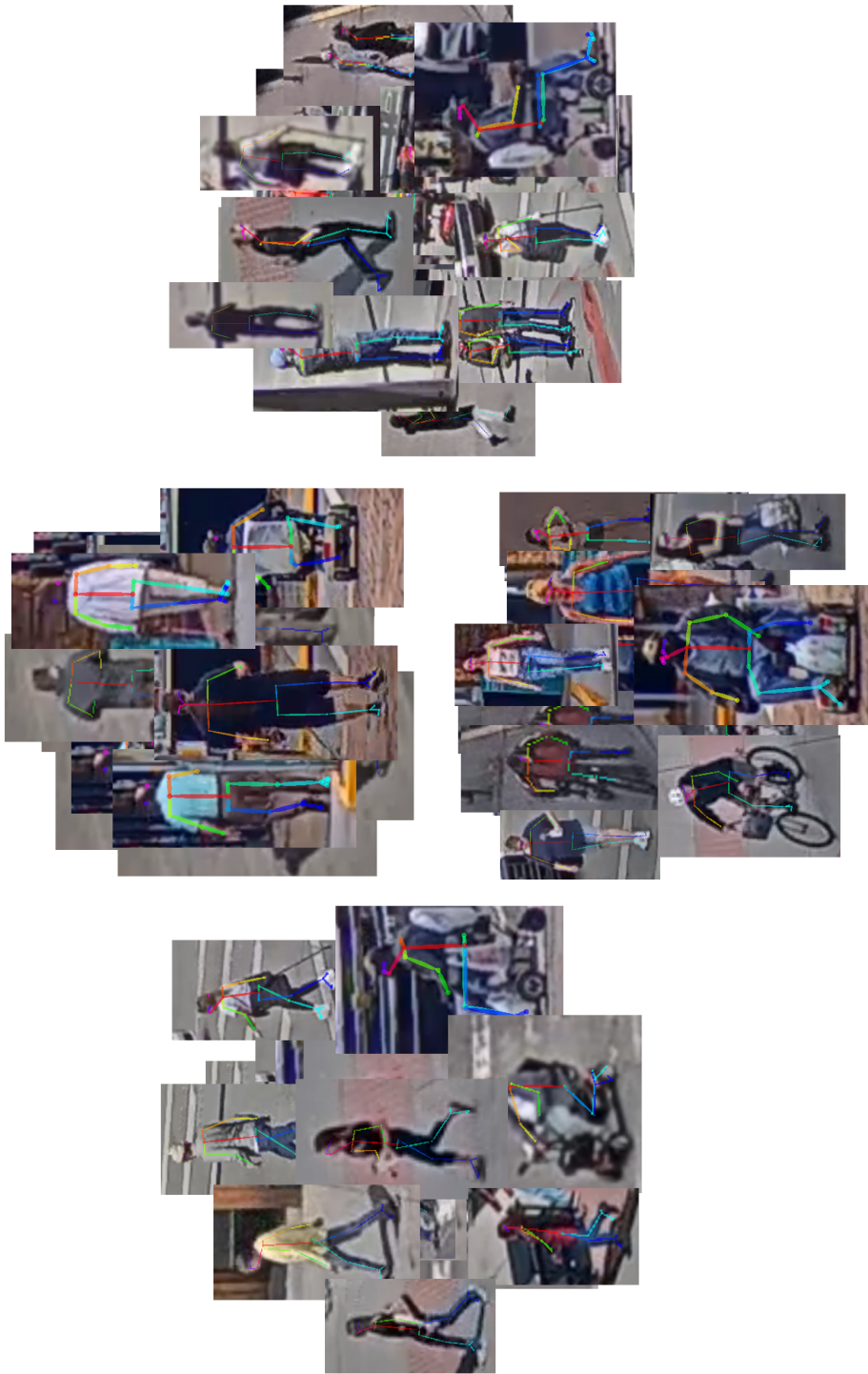
Figure 7.11: The pose direction estimation result visualization. All the input objects are calculated the \beta with four default cross directions under the related BEV plane. The visualization group is clustered to the belonging direction.
