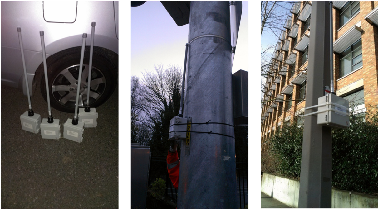
Figure 4-3: STAR Lab Bluetooth detectors (MACAD device) used in this study
