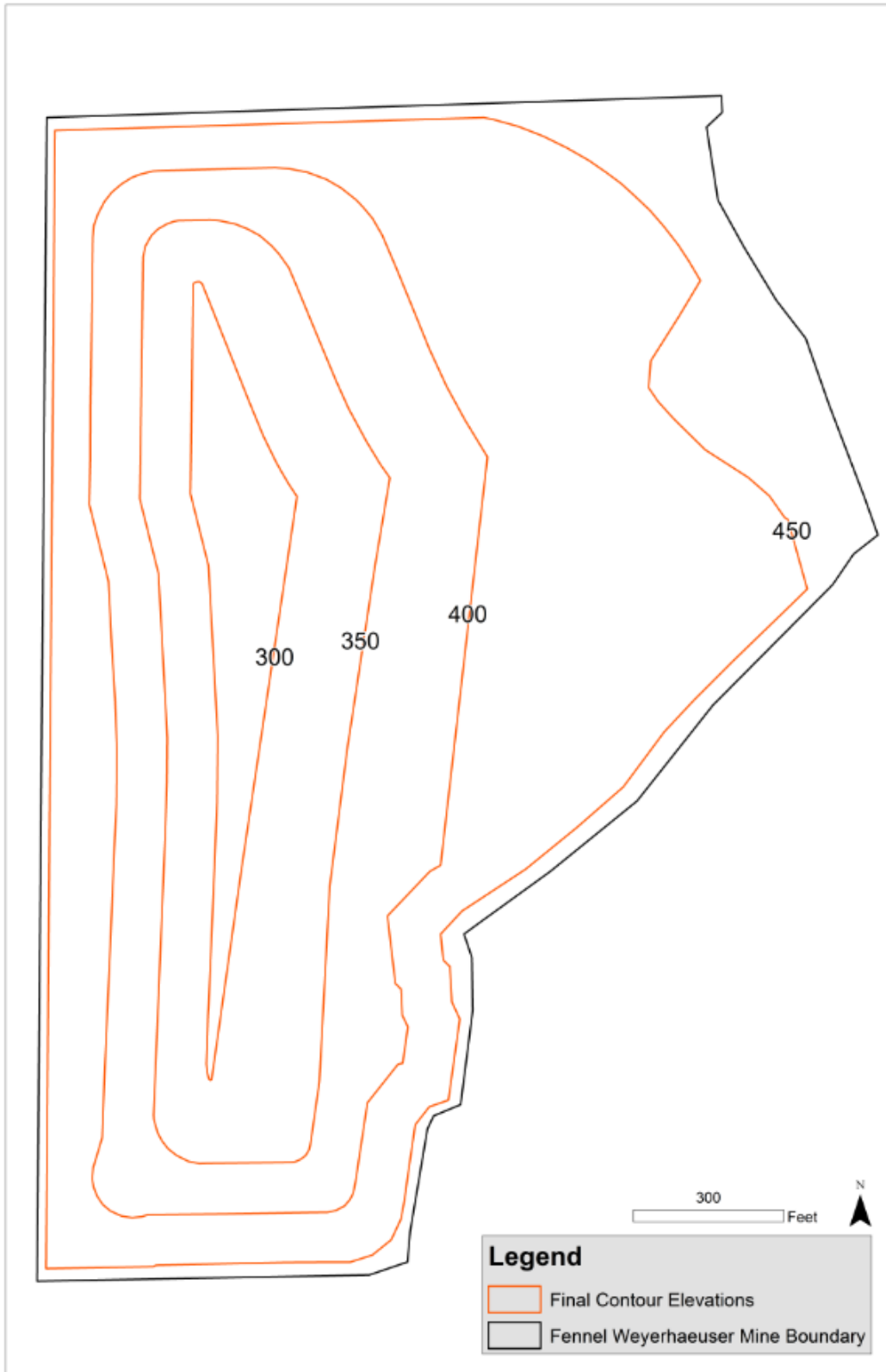
Figure 17: Final Mine Contours. The contours are based on the 2H:1V DNR slope requirements and AESI 2015 groundwater elevation along with the required groundwater buffer of 5ft.
