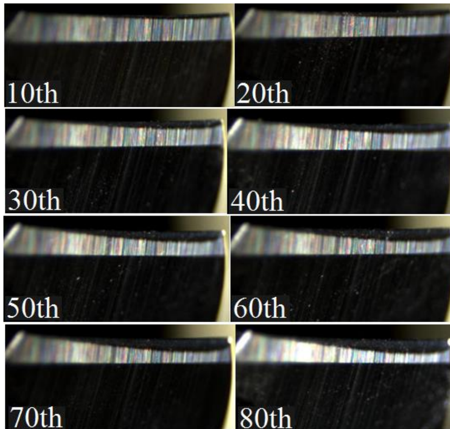
Figure 8.24. Representative optical image of the cutting edge from drilling Condition I
