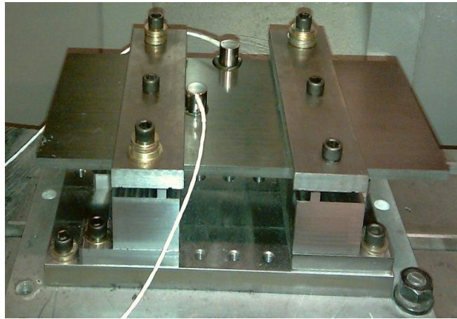
Figure 4.6. Optical image of AE sensor placement
