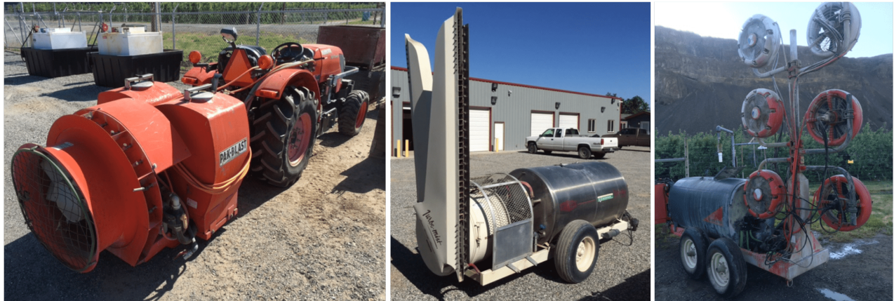
Figure 3.1: Images of Axial Fan Airblast (AFA), Directed Air Tower (DAT), and Multi-headed Fan Tower (MFT) sprayers (from left to right).
