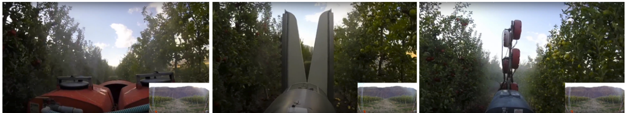
Figure 3.5: Tractor view of spray trials in research orchard blocks. Camera #2 was positioned on the seat of the tractor pulling the sprayer, facing backwards during the spray trials. Images are from the AFA, DAT, and MFT sprayers (from left to right).
