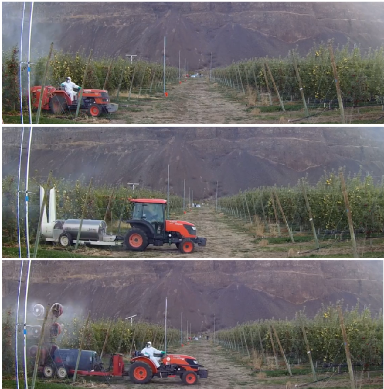
Figure 3.7: Side view of spray trials in research orchard blocks. Camera #3 was located approximately 10 m from the western edge between the sprayed and sampling fields (Figure 3.6), with a side view of the sprayers. Images are of the AFA, DAT, and MFT sprayers (from top to bottom).
